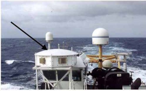
Figure 1. Electronically stabilized phased array 915-MHz antenna (arrow): NOAA research vessel Ronald H. Brown looking aft.
