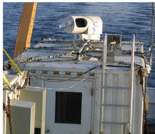
Figure 2. High Resolution Doppler Solid State Lidar (HRDL) system on board the NOAA research vessel Ronald H. Brown looking aft.
