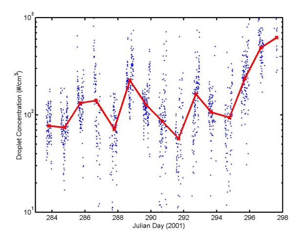
dropconcen\_time1. Cloud droplet concentrations computed from  $r_e$ , LWP, and cloud thickness. The dots are individual 5-min values; the red x's are daily medians. The rapid increase at the end of the time series is attributed to increased aerosol concentrations as the ship neared the coast of Chile.
