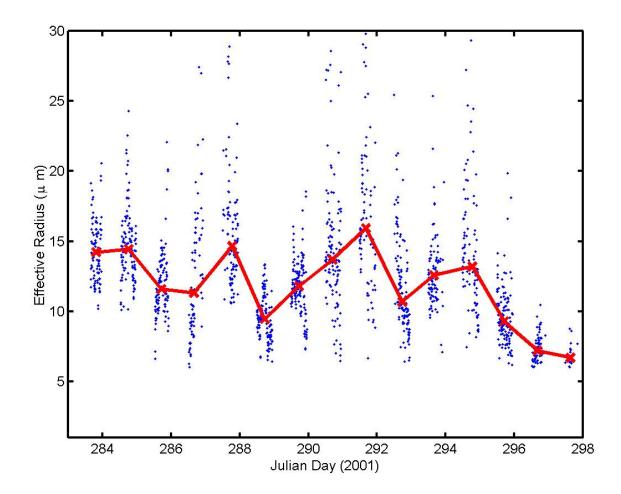
reffect\_time1. Time series of effective radius deduced from  $\tau$  and LWP. The dots are individual 5-min values; the red x's are daily medians. The rapid drop at the end of the time series is attributed to increased aerosol concentrations as the ship neared the coast of Chile.
