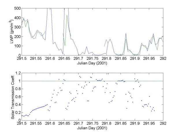
sol\_LP291. Time series of cloud LWP (upper panel) and solar transmission coefficient, Tr=Rsdm/Rsclear (lower panel). A value of Tr=1 implies clear sky conditions. Points exceeding one on this graph are caused by clouds in the field of view that do not block the sun's direct beam but reflect radiation to the sensor.
