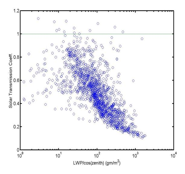
trans\_lwp1. Measured transmission coefficient as a function of LWP in the direction of the sun. Increasing values of LWP decrease the solar transmission, but once LWP exceeds about 100 gm/m², the effect begins to saturate.
