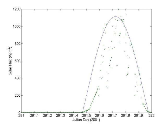
solclear291. Time series of measured downard solar flux, Rsdm (dots), and a model calculation of the expected solar flux for cloudless sky conditions, Rsclear (line).
