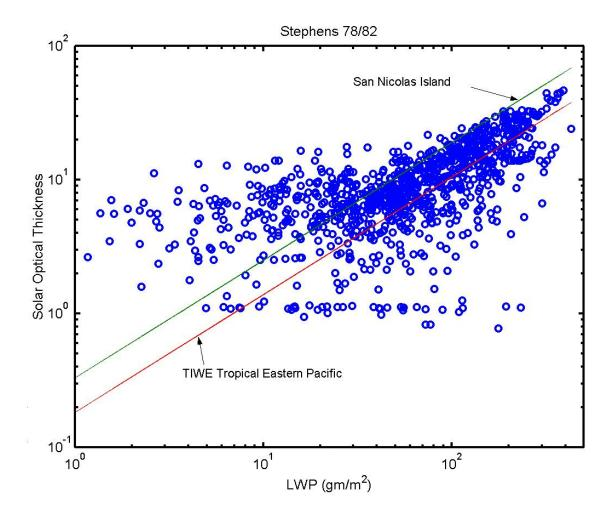
tau\_lwp1. Optical thickness computed from  $\mu$  and Tr using the model of Stephens (1978) as a function of LWP. The green line is a mean curve from measurements made at San Nicolas Island off the coast of California in 1987. The red line is from ship measurements made near the equator at 145 W longitude in 1992. These characteristic lines are typical of the kinds of relationships used in climate models.
