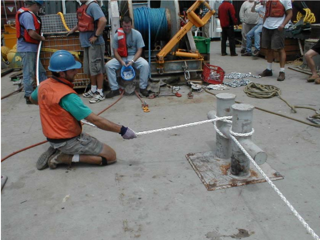
Figure 73: Position of the line handler and assistant.
