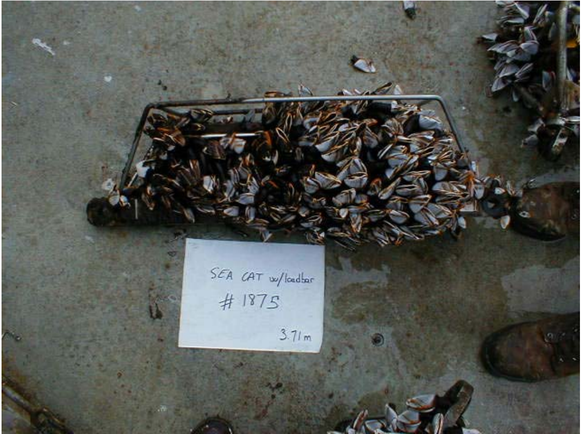
Figure 37: SEACAT instrument at 3.71 m depth.
