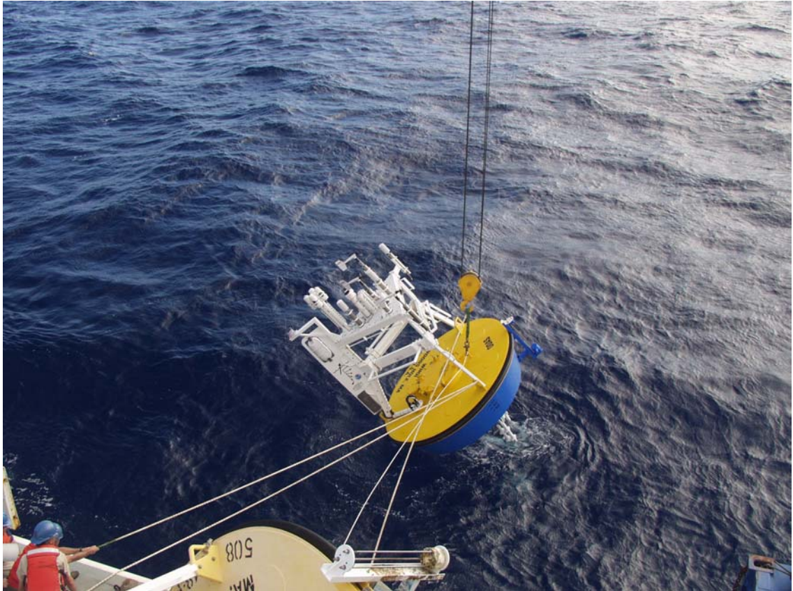
Figure 70: Three slip lines rigged on the discus to maintain constant swing control during the lift.
