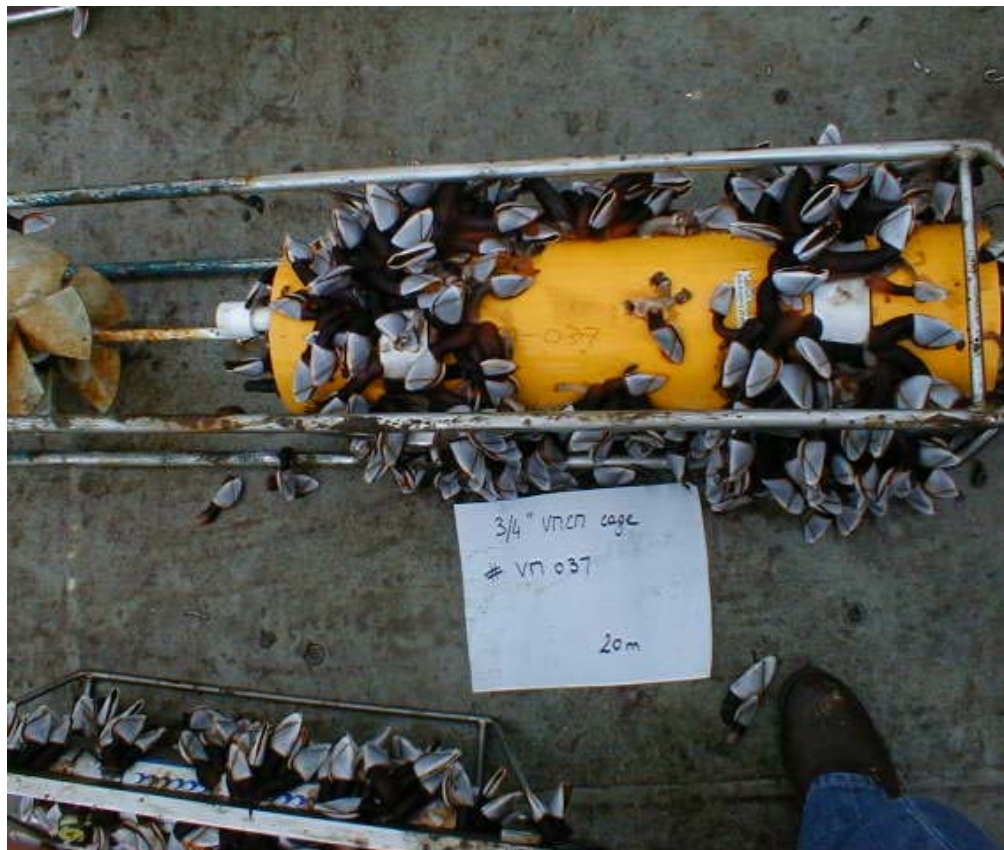
Figure 36: VMCM instrument at 20 m depth.
