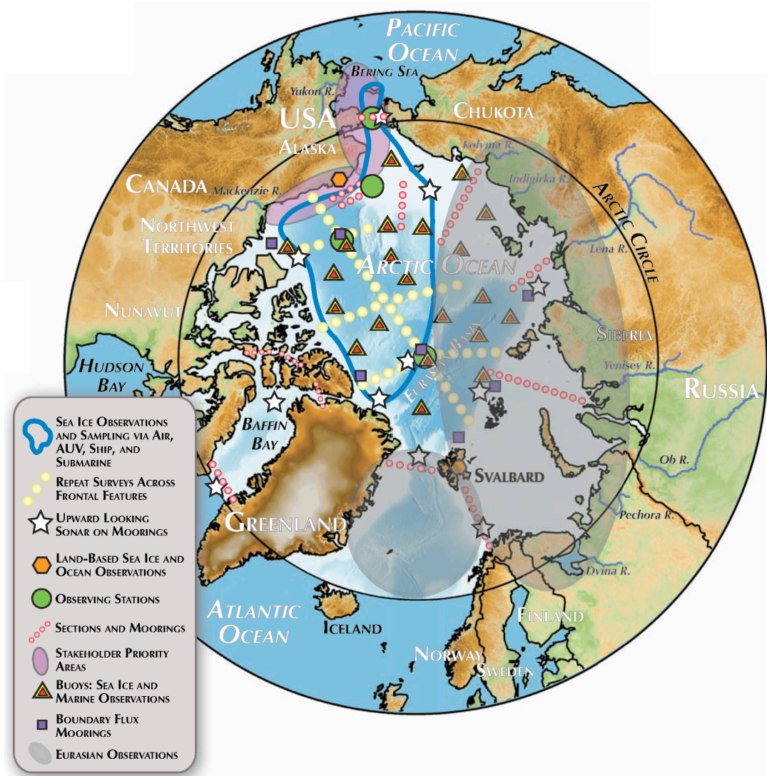
Figure 3. (from [20]) Priority areas for ocean and sea ice measurements. High priority areas include gateways for exchange between Arctic and Subarctic basins, major storage basins, the broad shelf-slope systems and sections across critical frontal regions. Many sites target long timescale change and sit far from centers of human activity, while others (pink shading) might deliver more targeted tactical information to stakeholders. Drifting autonomous assets (e.g., IBOs) would be distributed through the deep basin as depicted by the red triangles. Moorings and gliders monitor the gateways and shelf-slope regions (red circles and grey squares) while gliders conduct repeat occupations of cross-basin sections that span key frontal features (yellow circles).
