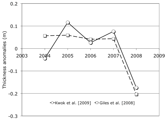
Figure. 6 Comparison of the thickness anomalies derived from the Envisat radar altimeter [12] and the ICESat lidar. (after [2])
