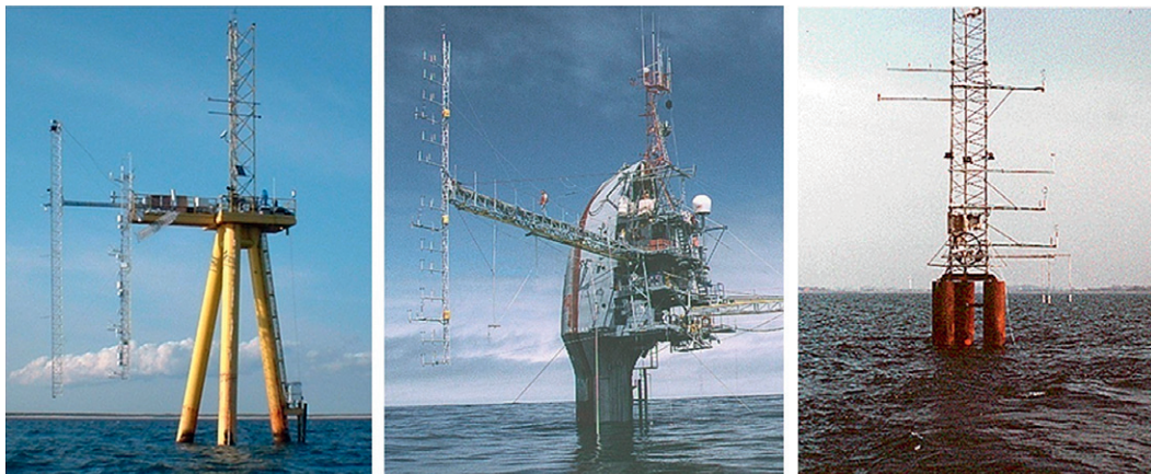
FIG. 4. The three platforms used to directly measure flux–profile relationships during the CBLAST, MBL, and RASEX programs. (left) The ASIT tower used in CBLAST where the profiling mast is at far left and the mast holding the fixed sensors is nearer the platform. (middle) The R/P FLIP used in MBL and (right) the tower used in the RASEX program.
