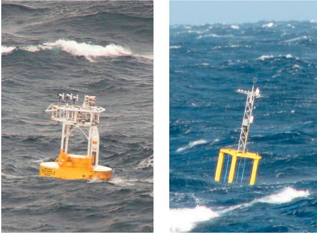
FIG. 1. (left) The 2.7-m foam-hull buoy and (right) ASIS platform used during the CLIMODE program to provide DC estimates of the momentum and heat fluxes. The moored buoy was successfully deployed for 15 months in the Gulf Stream, while the ASIS was deployed for 14 days.
