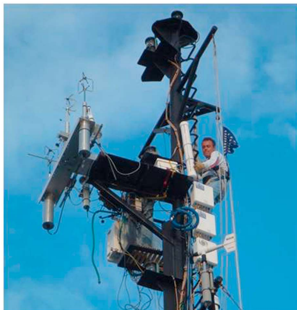
Figure 4. (left) Installation of the fast sensor instrumentation on jackstaff. The central sonic anemometer was positioned 1.6 m forward of the main mast. (right) Close-up of sonic anemometers, fast humidity sensors, and mean T/RH sensors on the jackstaff of the NOAA ship Ronald H. Brown for SO GasEx. The PSD sonic is in the center, and the DCFS sonics are port (left in the photograph) and starboard (right in the photograph). The sleeved fast sample LI-7500 is the unit on the right with the large blue ventilation system. The three open path units are on the left. Each sonic is mounted to its own motion-measuring system.
