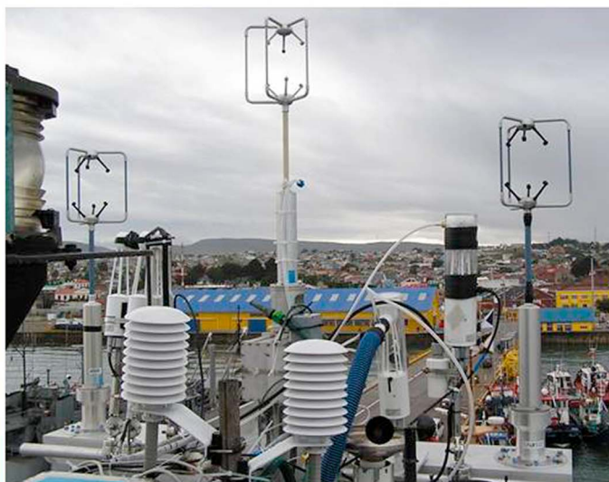
Figure 4. (left) Installation of the fast sensor instrumentation on jackstaff. The central sonic anemometer was positioned 1.6 m forward of the main mast. (right) Close-up of sonic anemometers, fast humidity sensors, and mean T/RH sensors on the jackstaff of the NOAA ship Ronald H. Brown for SO GasEx. The PSD sonic is in the center, and the DCFS sonics are port (left in the photograph) and starboard (right in the photograph). The sleeved fast sample LI-7500 is the unit on the right with the large blue ventilation system. The three open path units are on the left. Each sonic is mounted to its own motion-measuring system.
