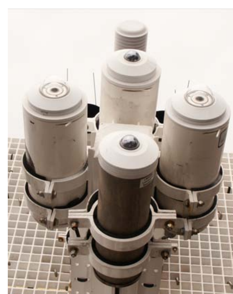
Figure 3. A buoy radiometer assembly. For redundancy there are two Eppley PIRs (reflective domes) and two PSPs (clear domes) mounted on a buoy tower.
