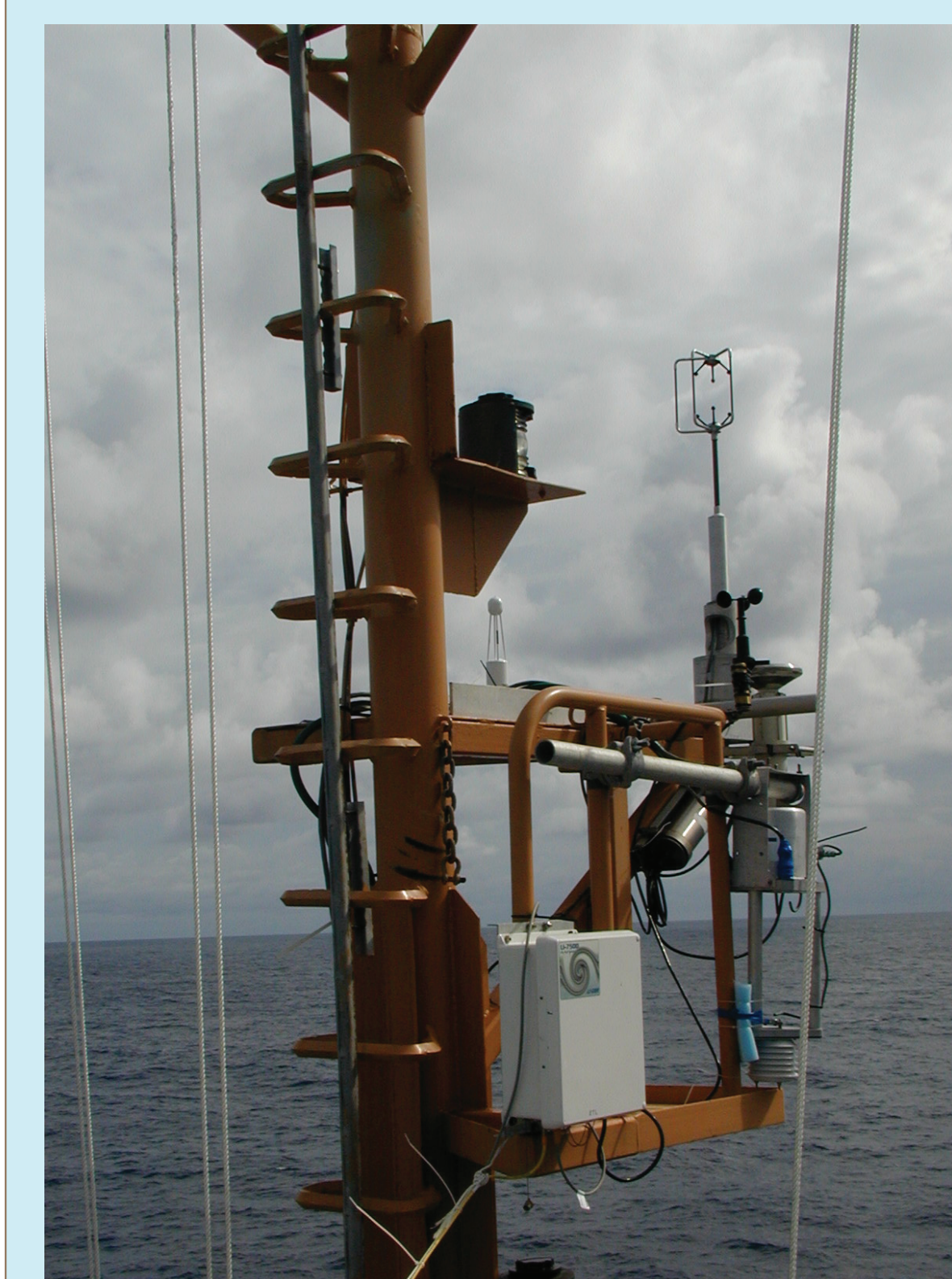
R/V Ronald Brown Flux System. Wireless transmitter are connected to: Sonic, Licor, Laser wave gauge
