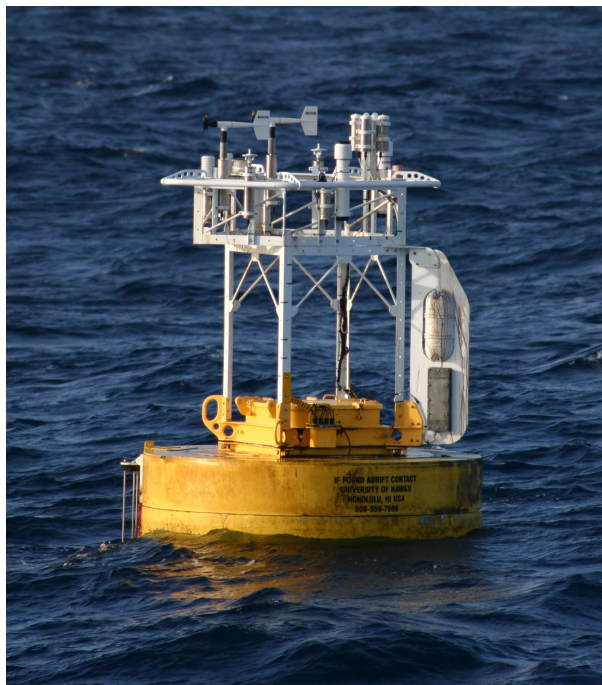
Fig. 10. Surface buoy, showing wind-orienting vane to keep sensors on the upwind face, wide separation of sensors, and placement of radiometers as high as possible.
