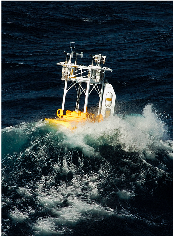
Fig. 1. Surface buoy deployed in 2005–2006 in the core of the Gulf Stream, equipped with three propeller-vane anemometers and a sonic anemometer for the DC method. (Whelan, S., WHOI).
