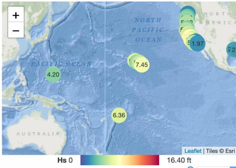
**Figure 5.** Locations of CDIP buoys with shading indicating significant wave height, Hs.
