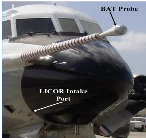
Figure 6. Location of the BAT turbulence probe and LICOR fast response humidity probe on the WP-3D aircraft.
