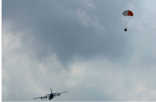
Figure 3. Deployment of a drifting buoy package from an AFRC WC-130J aircraft.
