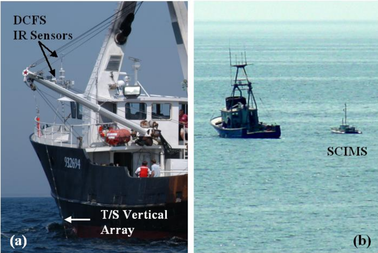
Figure 5. a) Instrumentation deployed on the Nobska during the 2003 IOP. Bow instrumentation included a direct covariance flux system and IR radiometers. The boom supported an array of temperature/salinity sensors for high-resolution vertical profiles. b) Photo taken from the Air-Sea Interaction Tower at MVCO of the SCIMS catamaran accompanied by R/V Asterias during a southeasterly survey transect on August 15, 2003. Numerous banded surface film features (light areas) evident in the field of view were quantified by SCIMS instrumentation.
