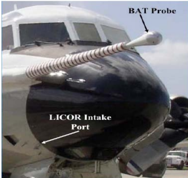
NOAA ARL Best Atmospheric Turbulence (BAT) Probe 11/13/2009
