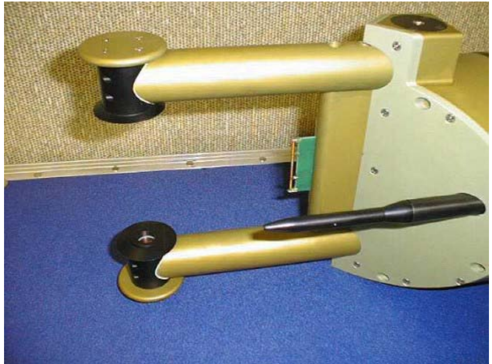
Droplet Measurement Technology Drizzle and Sea Spray Probe
