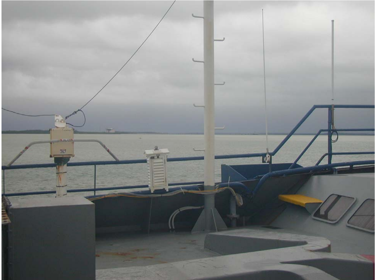
Figure 3.3. A more usual type of screen to house the wet and dry bulb thermometers read hourly by the bridge officers. It is also well exposed, and all four sides are louvered to allow free airflow to the thermometers.
