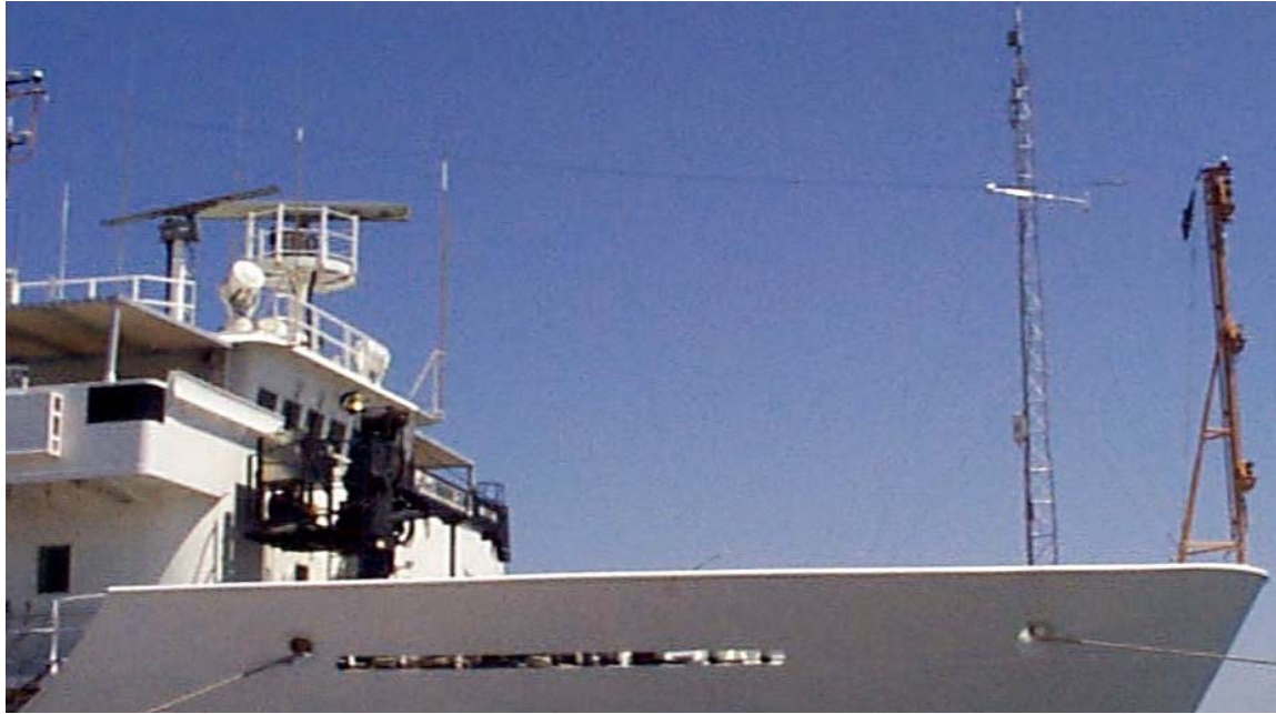
Figure QR2. Guyed mast installed on foredeck for good exposure of meteorological instruments.
