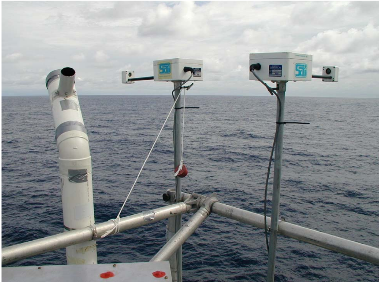
Figure 3.6 Example deployment of optical rain gauges. A pair of sensors is mounted with their axes oriented at 90° to each other. This geometry helps with the wind correction procedure.
