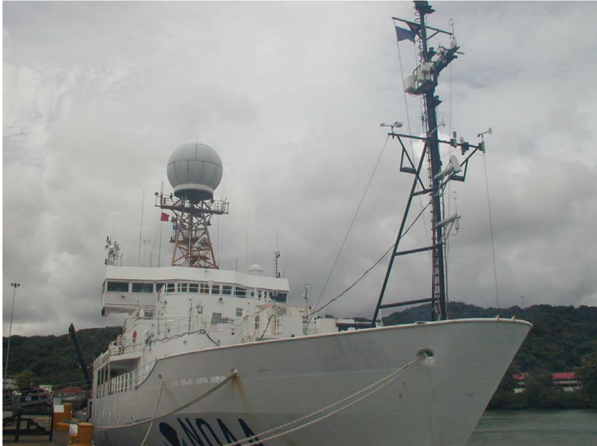
Figure 9.1 Meteorological instruments on the foremast of the NOAA ship Ronald H. Brown ; a) below the upper cross-arm is a covariance package. The sensor of the sonic anemometer is well exposed, although the instrument boxes below and behind it represent a greater obstacle to airflow than is desirable; b) close-up of the bulk flux instrument package. From left to right on crossarm: optical rain gage; T/RH sensor with forced ventilation; second T/RH sensor in naturally ventilated screen; siphon rain gage; propeller anemometer and wind vane unit. Below these instruments can be seen a laser wave-height sensor aimed forward of the bow and a second sonic anemometer.
