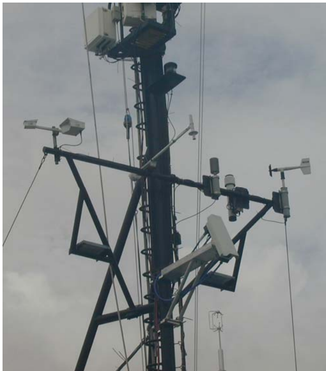
Figure 9.1 Meteorological instruments on the foremast of the NOAA ship Ronald H. Brown ; a) below the upper cross-arm is a covariance package. The sensor of the sonic anemometer is well exposed, although the instrument boxes below and behind it represent a greater obstacle to airflow than is desirable; b) close-up of the bulk flux instrument package. From left to right on crossarm: optical rain gage; T/RH sensor with forced ventilation; second T/RH sensor in naturally ventilated screen; siphon rain gage; propeller anemometer and wind vane unit. Below these instruments can be seen a laser wave-height sensor aimed forward of the bow and a second sonic anemometer.
