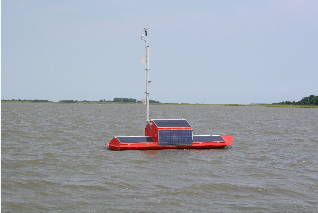
Figure 20: Field Deployment of the Ocean-Atmosphere Sensor Integration System (OASIS) Autonomous Surface Vehicle (ASV). The platform was developed under joint NASA-NOAA funding and commercialized through a NASA-SBIR award. It is being marketed commercially through Pacific Gyre, Inc.
