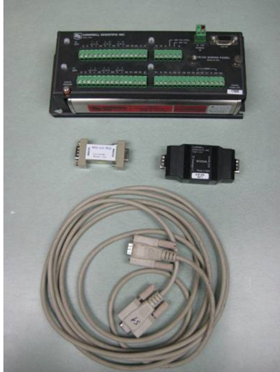
CR10x Datalogger (Serial #: X 34172) & Datalogger Adapters
