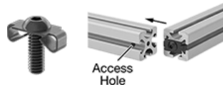
Concealed (Tap one hole to install the connector and drill one access hole in the mating rail to secure the connection.)
