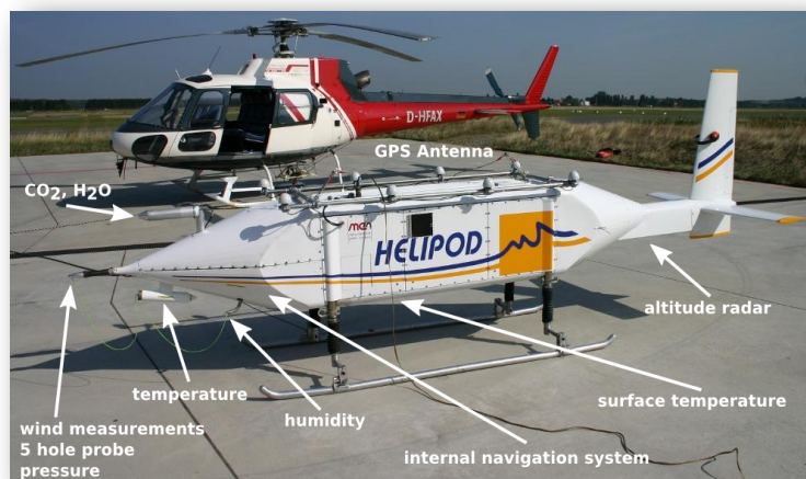
Fig. 3.2: The Helipod and its instrumentation
