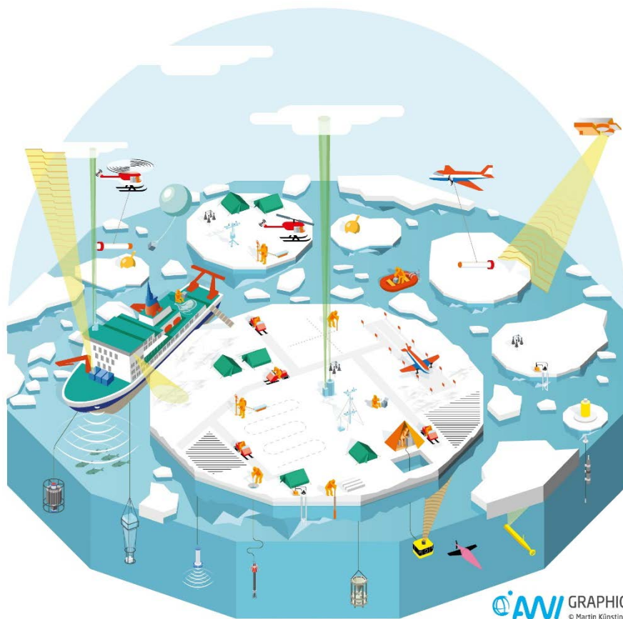
Fig 1.1: Illustration of the layout of the main elements of the MOSAIC experiment: Polarstern is moored to the central observatory and it is surrounded by the distributed network and connected to the larger scales through airborne measurements, other research vessels and satellites. The illustration of the ice camp sketches the different installations and research areas on, above, and under the sea ice. (Figure: Alfred Wegener Institute, Helmholtz Centre for Polar and Marine Research (AWI)/Martin Künsting CC-BY 4.0).
