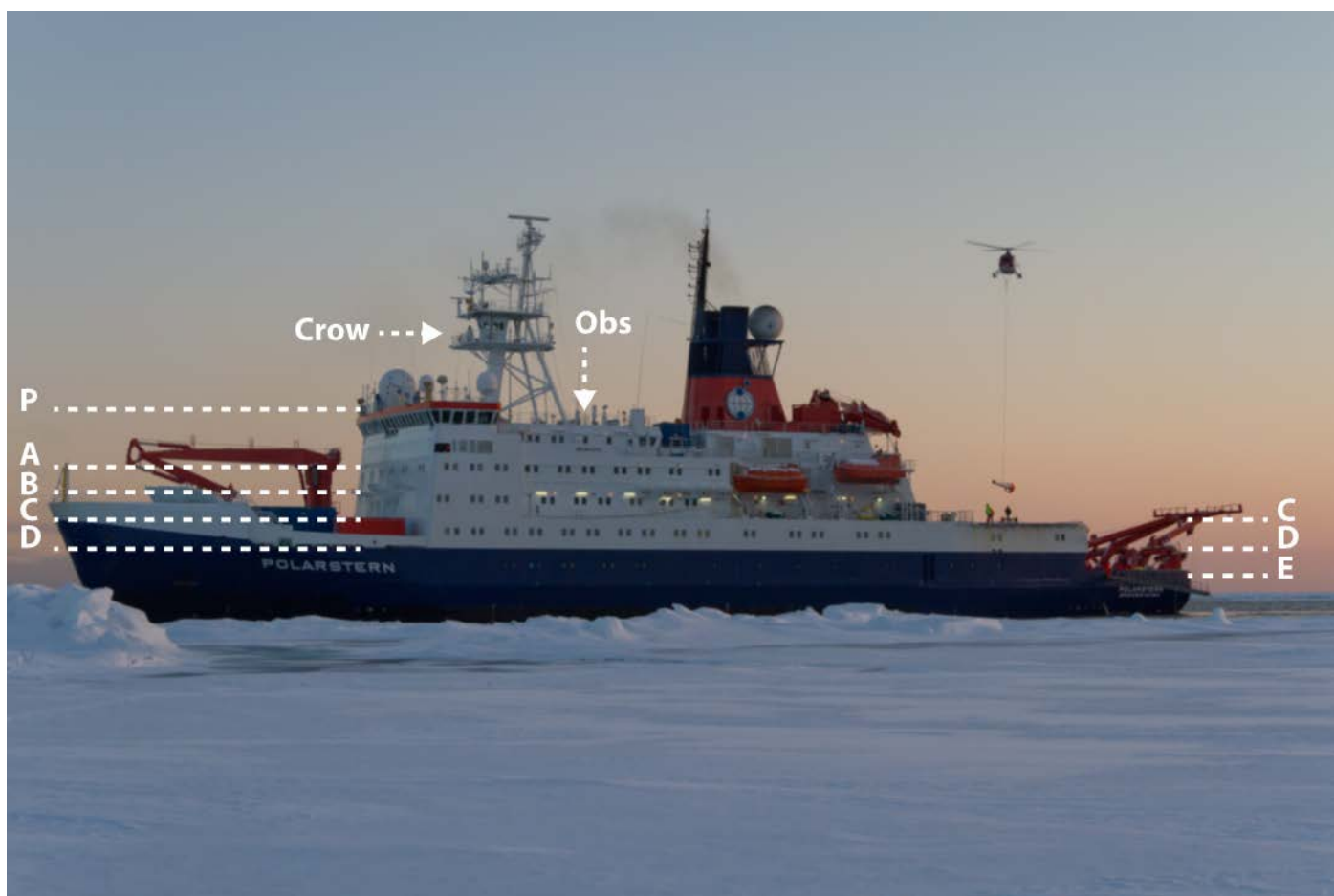
Fig. 3.2: Photo of Polarstern in sea ice with a helicopter taking off for a measurement survey. Letters name the decks on board: E-Deck includes the working deck in the aft, D-Deck is the bottommost white deck, C-Deck hosts the helicopter platform, A-Deck is directly under the bridge, and P-Deck (German: Peildeck) on top of the bridge with the Observation (Obs) deck behind it and some steps lower. The Crow's nest (Crow) is the highest observational platform.
