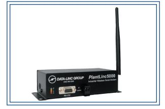
PlantLinc<sup>™</sup> 5000 Industrial Wireless Serial Modem (model PLR5000) is an industrial serial RS232 radio modem designed for cost-effective, short-range PLC communications up to 4 miles. It operates in the license free 902-928 MHz band and uses frequency hopping transmission techniques for excellent reliability in noisy plant environments. It is a cost effective alternative to cable installation, trenching and leasing expensive phone lines to remote locations.
