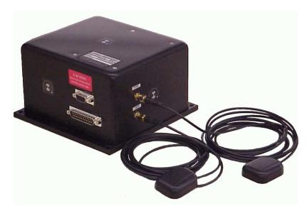
set of three outputs measure the acceleration aligned with an earth-level coordinate system. This allows forward and lateral acceleration measurements that are essentially free of gravity influences. The triaxial sensor set allows software alignment of sensors, greatly reducing any alignment errors. The serial interface is highly configurable and provides access to almost all operational parameters.
