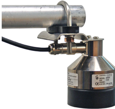
FIGURE 7-3. SR50A Mounted to a Crossarm via the 19517 Mounting Kit
