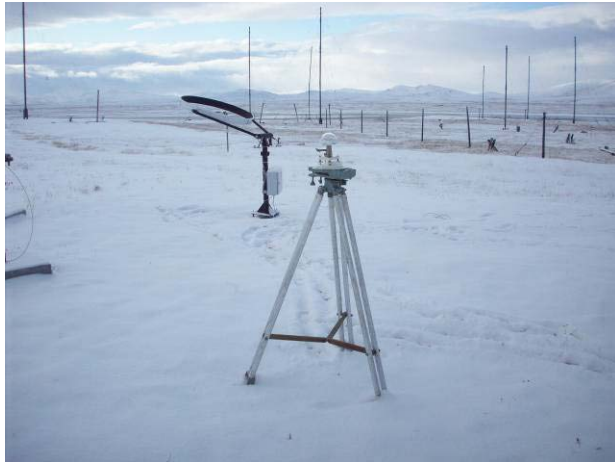
Figure 2.3: Russian sensors for measurement of total and diffused solar radiation, installed at the Hydrometeorological Observatory Tiksi (left) in October 2009 and an example of real-time data being received at the AARI Tiksi data center in St Petersburg, Russia (right).
