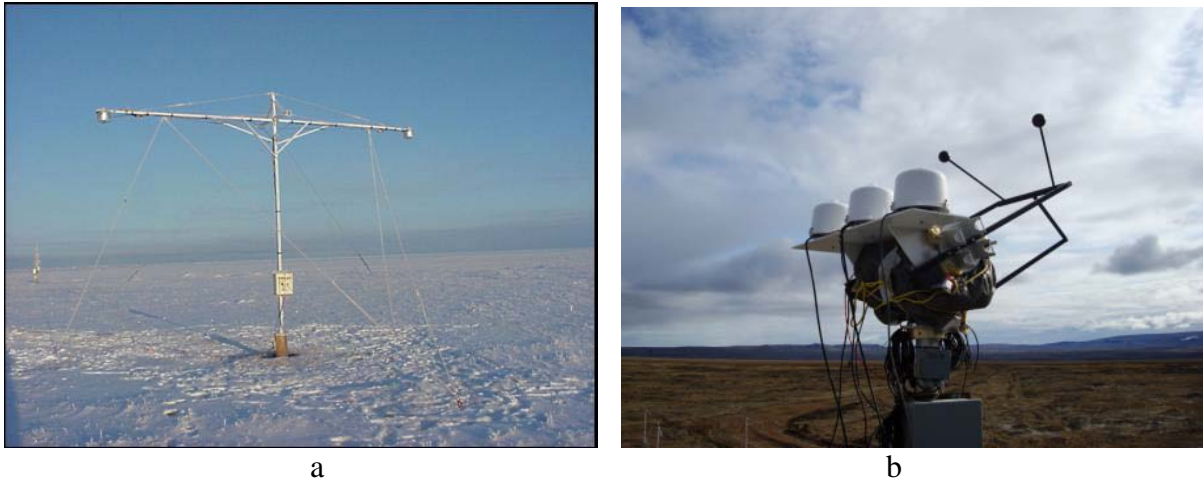
Figure 2.4: (a) BSRN Albedo rack with downward looking radiometers (b) BSRN upward looking radiometers and solar tracker
