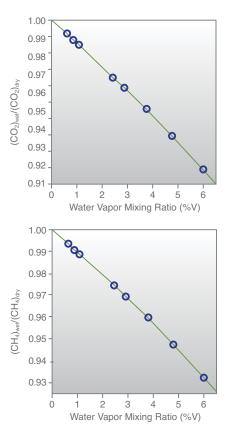
Mixing ratios for carbon dioxide and methane are only meaningful when extrapolated back to dry-gas conditions. Picarro's G2301 analyzer enables you to measure dry-gas mixing ratios for carbon dioxide and methane directly inthe wet gas stream. Only Picarro includes automated water vapor corrections which have been independently validated by top labs: NOAA, MPI, LSCE.
