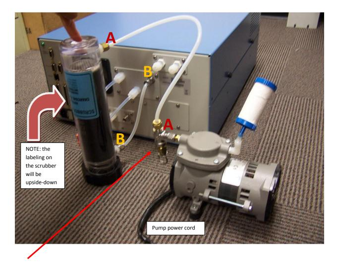
NOTE: Make sure that the connection to the external pump is connected as pictured above; Notice that the downward facing part of the "T" has a ring connected to it that is loosely attached to let excess pressure escape from the pump. IF these connections are not connected as pictured above, then remove and re-connect the tubing so that it IS connected as pictured above.
