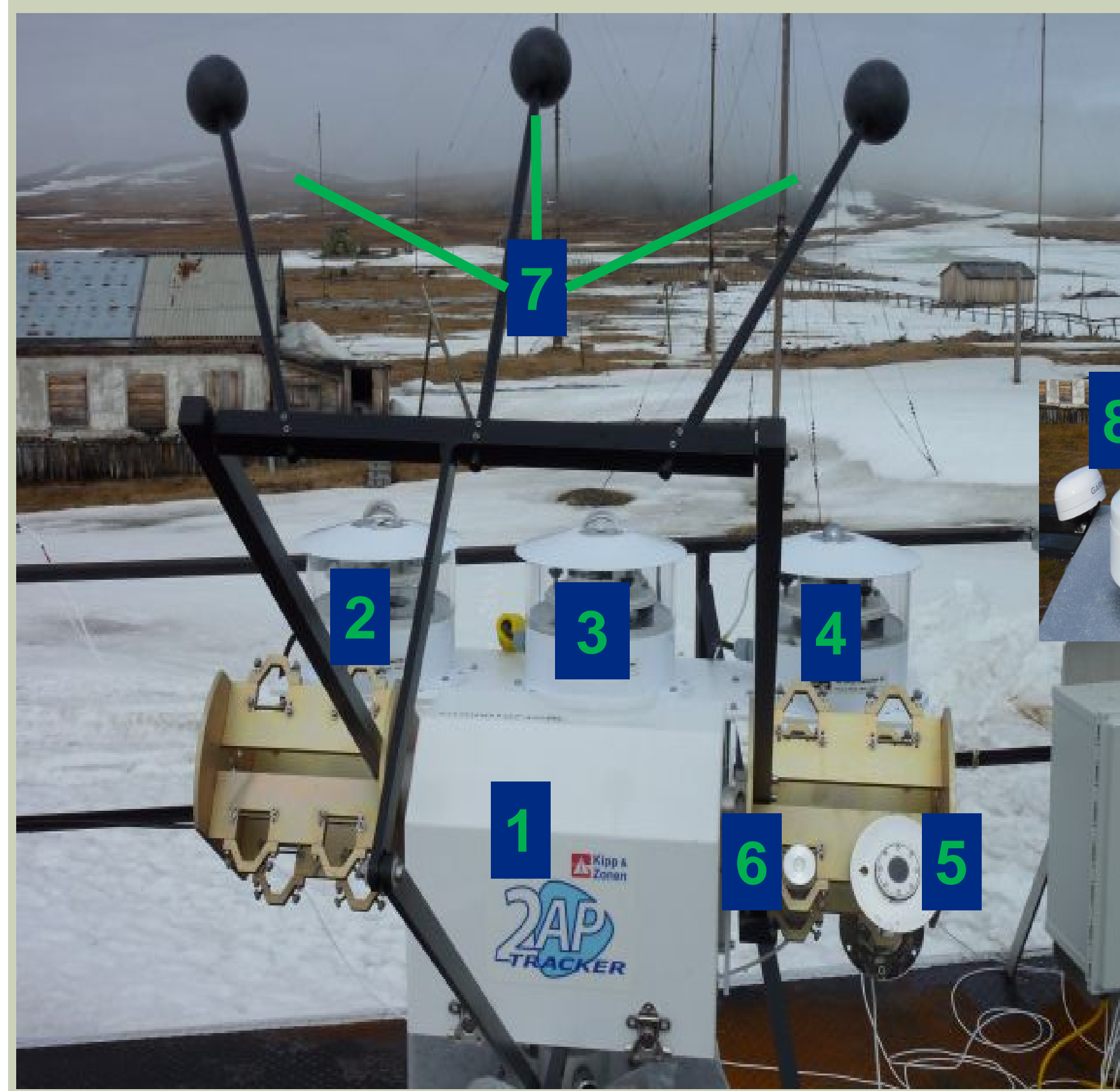
1: Kipp&Zonen 2AP tracker 7: Radiometer Shade Balls 6: Sun Sensor Tracker
