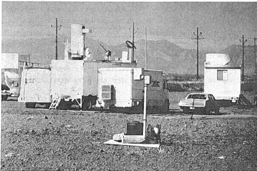
Figure 8.2b.--The WPL pulsed-lidar system deployed at PHOENIX. The all-sky camera is in the foreground. Auxiliary photometers are visible on top of the trailer. The TPQ-11 radar is at the right.
