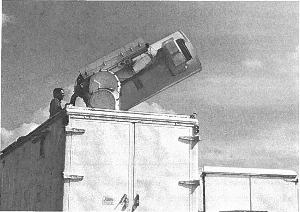
Figure 3.1. Lidar system. The telescope with laser and detector mounted astride scanned in elevation angle at several azimuth directions downwind of the source. The observer disabled the laser whenever an airplane approached the laser beam. When not operating, the scan assembly retracts into the semitrailer, which also contains workbenches and storage space. The operator's console and computer data acquisition system are contained in the vehicle on the right.
