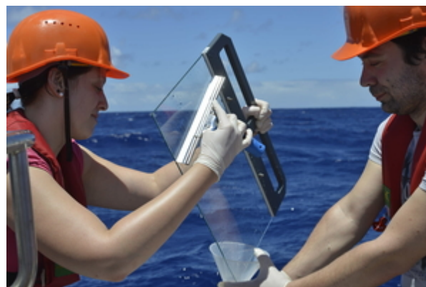
Figure 3: Sampling of the ocean surface film layer from a zodiac. © Hartwig Deneke, TROPOS.
