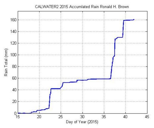
Figure 6. Time series of accumulated rainfall for CALWATER2. This time series is the consensus mean from six rain gauges.
