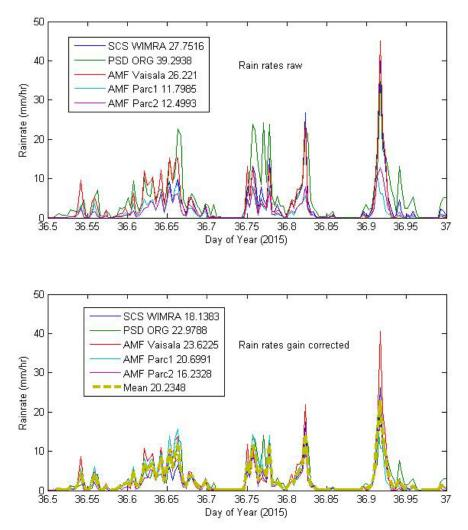
Figure 7. Time series of rain rate for 12 hours on Year day 36. Upper panel is raw rain rate from 5 gauges. The lower panel is the rain rate from the 5 gauges after gain correction. The heavy line is the mean of the 5 corrected gauges.
