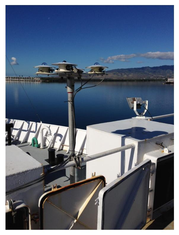
Figure 2. PSD PIR and PSP radiative flux sensors on 02 deck.
