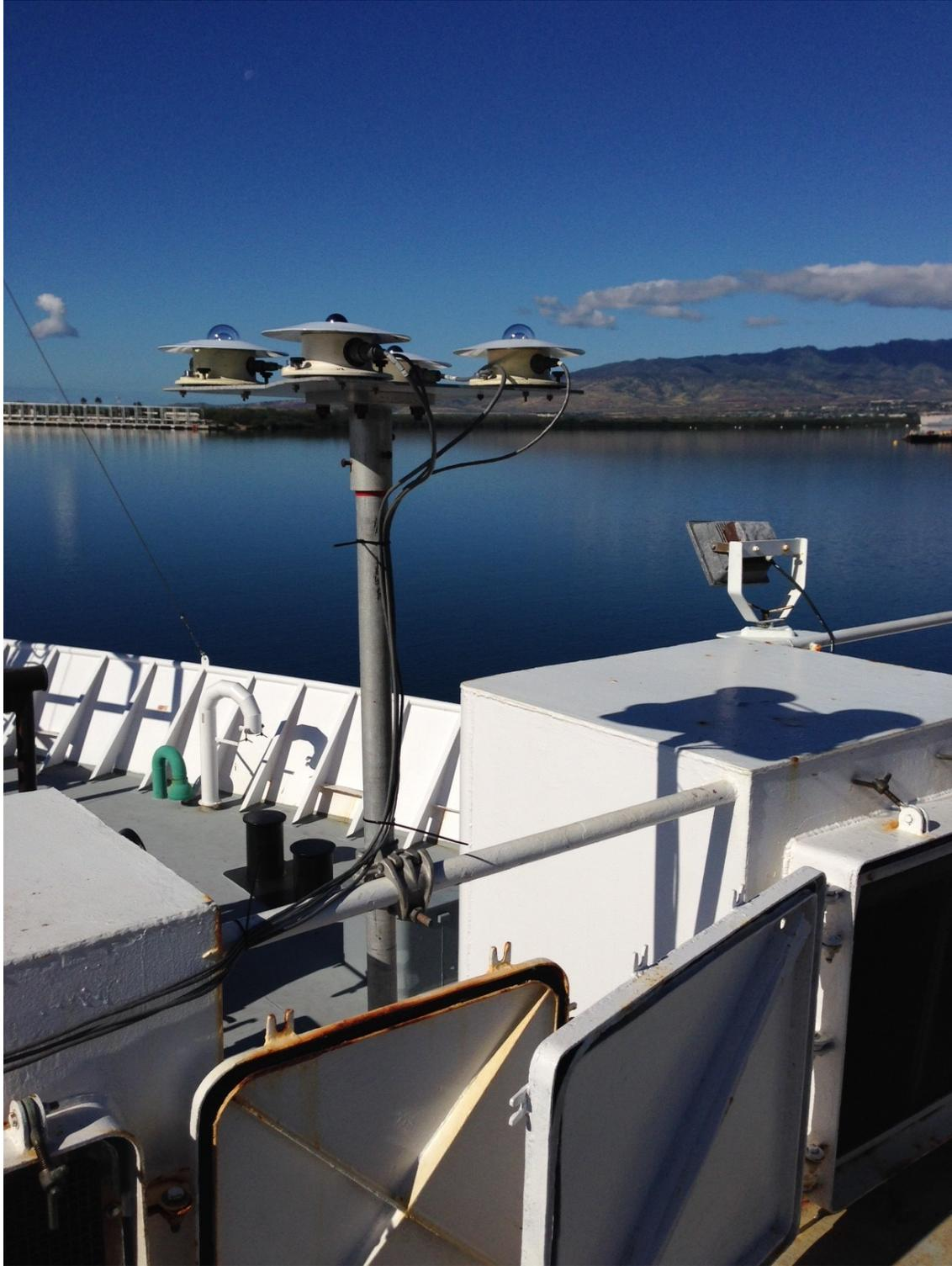
Figure 2. PSD PIR and PSP radiative flux sensors on 02 deck.
