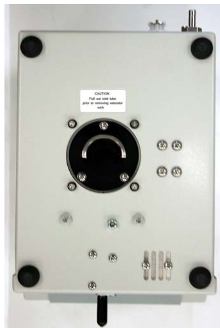
Figure 3-5 Bottom Panel Showing Removable Saturator Base
