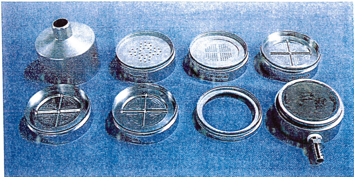
Figure 2. Model 130 High-Flow Impactor disassembled
