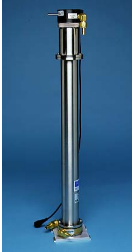
Figure 4-1 Model 3081 Long Differential Mobility Analyzer
