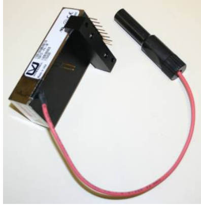
Figure 6-12 Positive High-Voltage Controller
