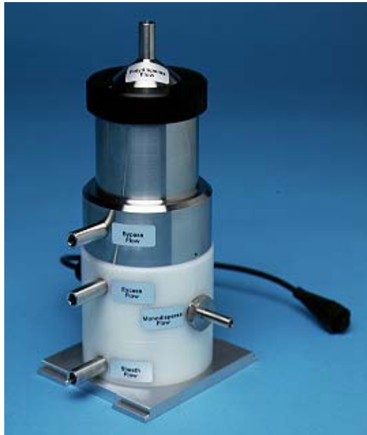
Figure 4-3 3085 Nano Differential Mobility Analyzer
