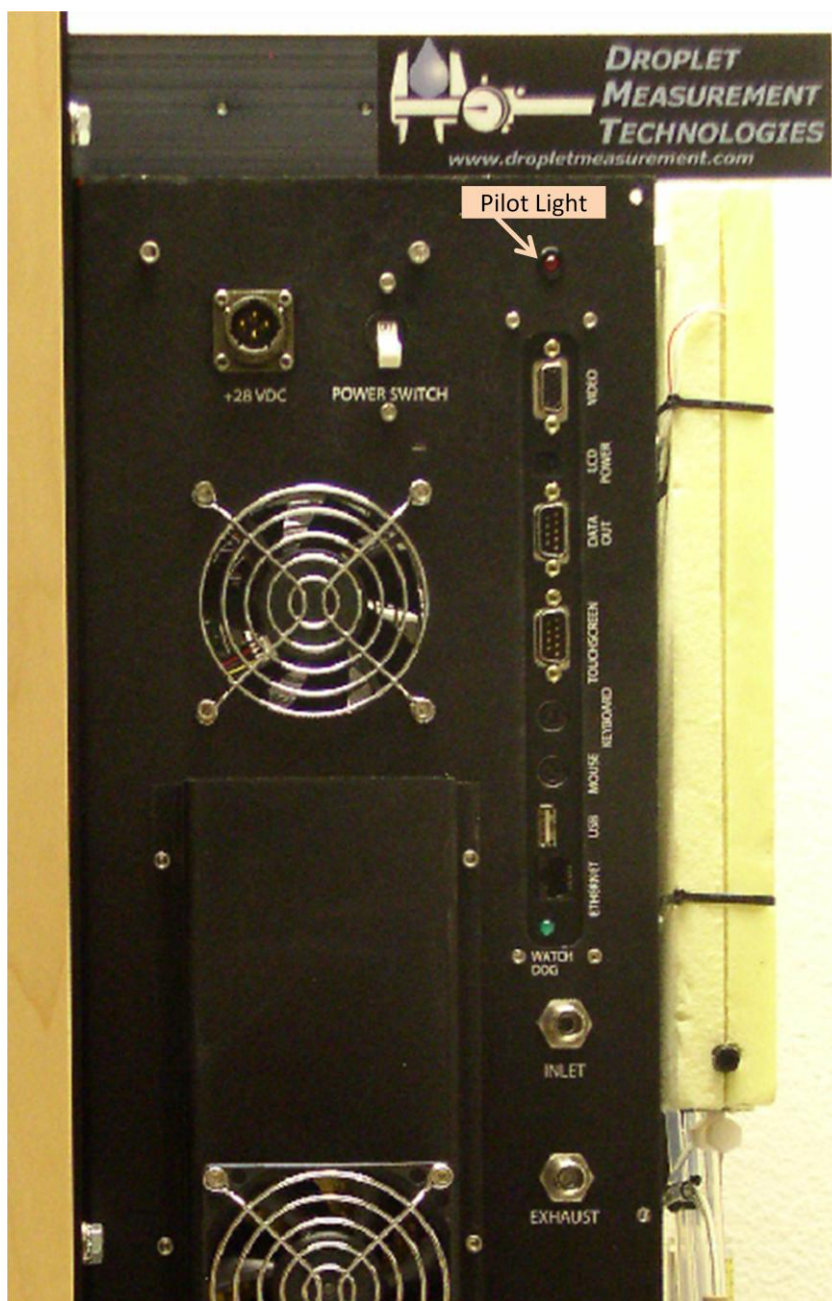
Figure 9: Location of Power, Communications, Sample and Exhaust Connections
