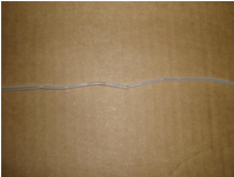
Figure 22: Typical Bad Membrane. Note the kinks and flat spots.
