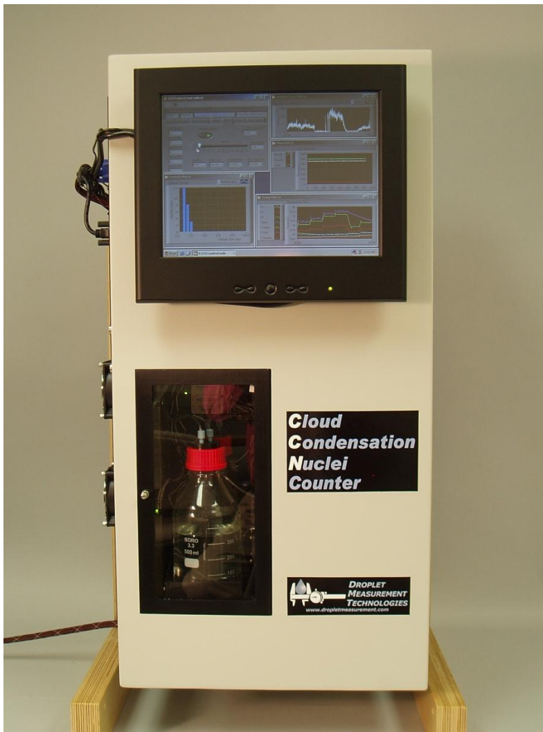
Figure 1: CCN Counter with Front-Mounted Touch Screen
