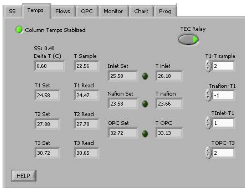
Figure 27: Temperature Tab Screen Showing Temperature Set Points and Read-Outs the CCN Temperatures
