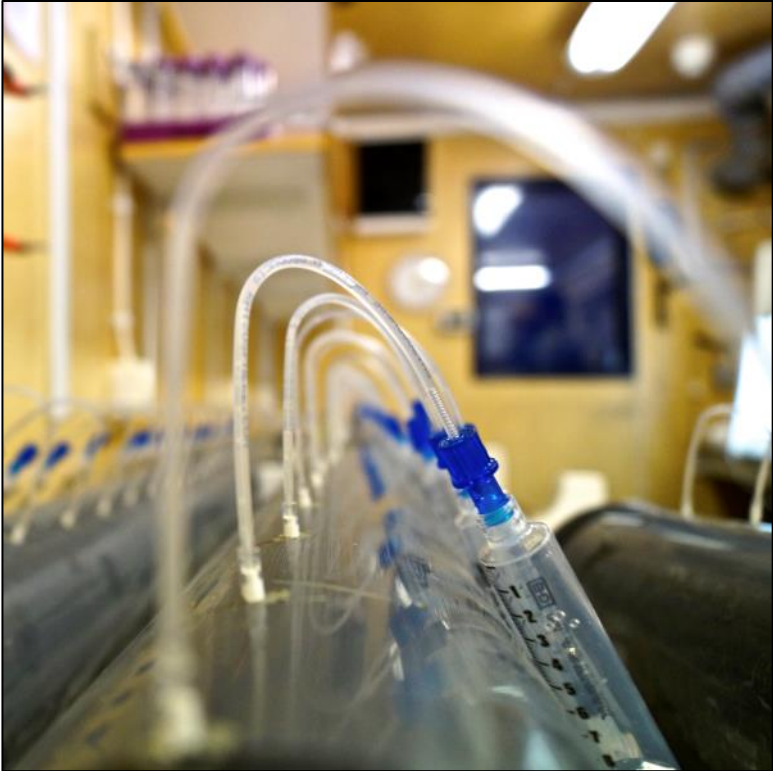
Figure CP-2: Rhizon samplers under negative pressure sampling water from a gravity core. The rate of sampling varied between Rhizons. The sampling times are given in Table CP-1. Photo Pedro Preto
