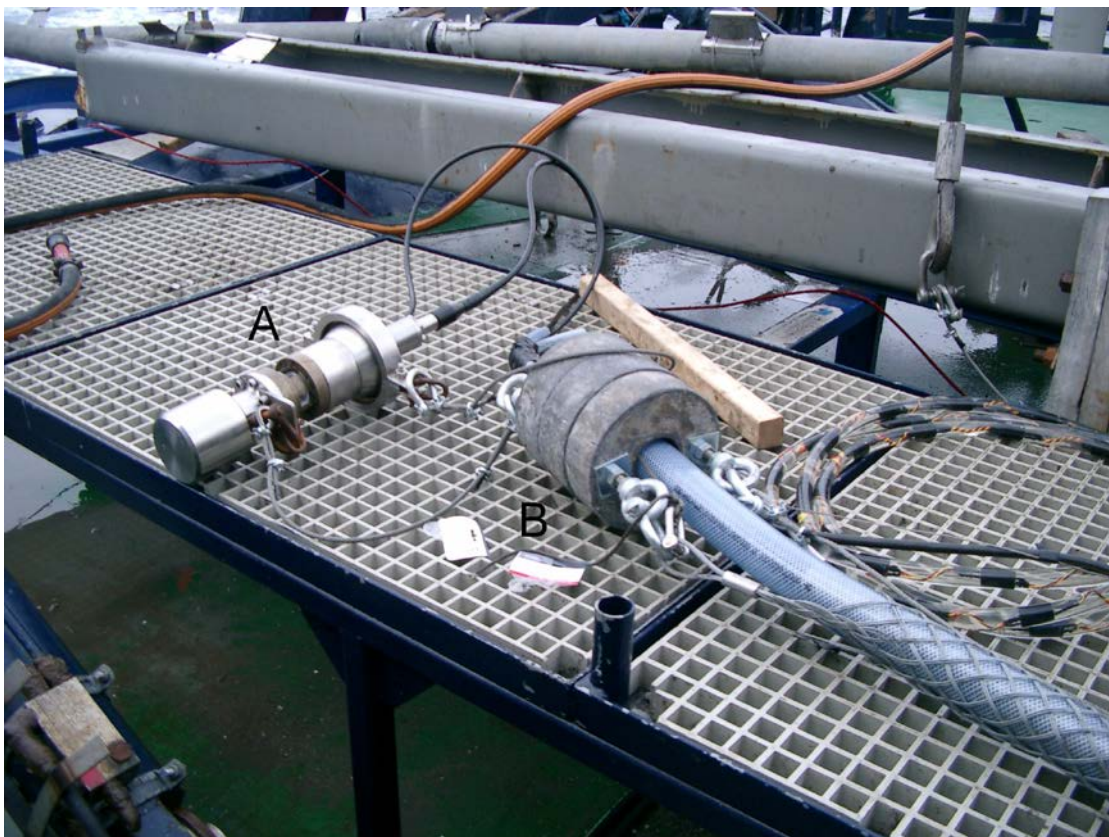
GM-9: The PAR-1600 airgun equipped with a 40 cubic inch (~0.66 liter) chamber used as seismic source (A) and the depressor weight (B) at the lower end of a plastic hose used to protect signal cables and air hose.
