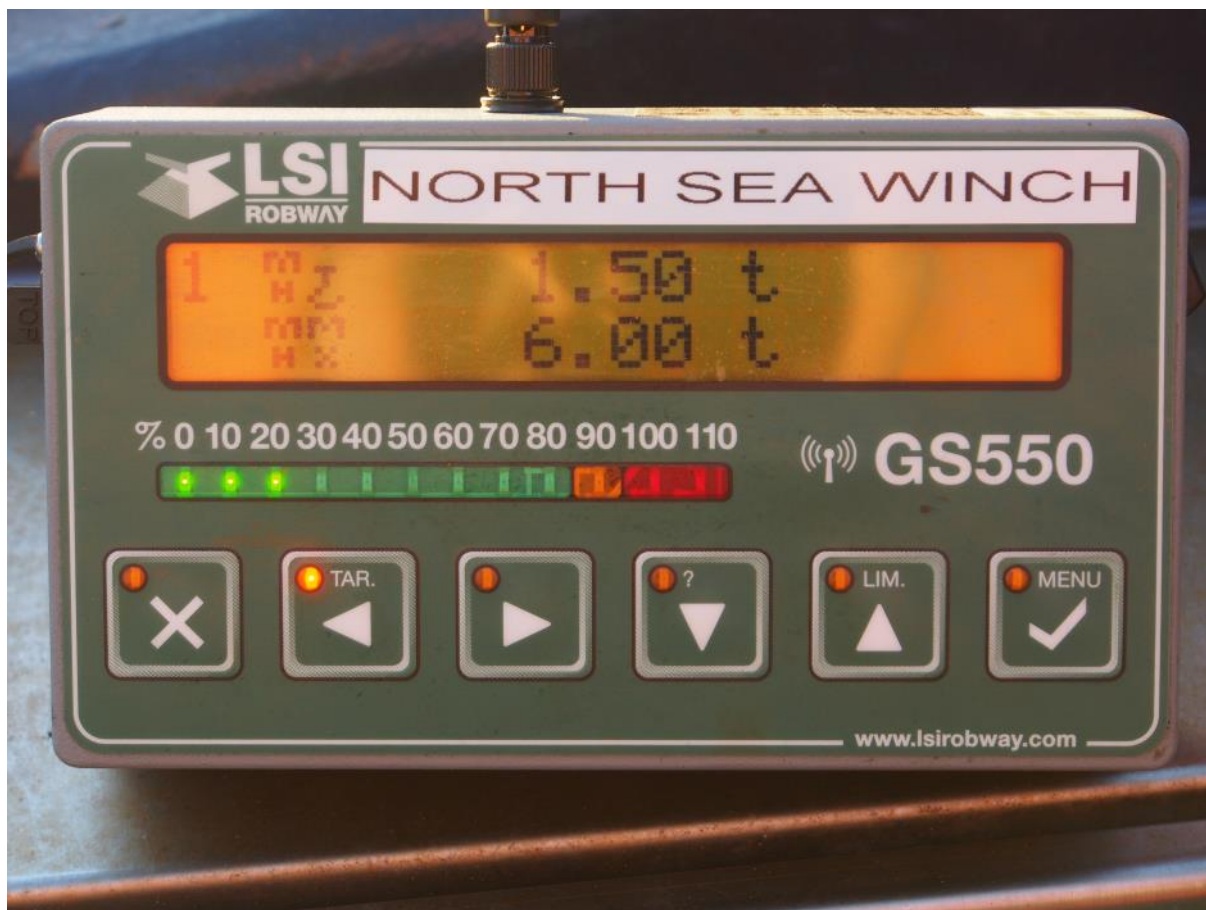
Figure SC-9: Remote display showing load and wire out of the NorthSea winch.
