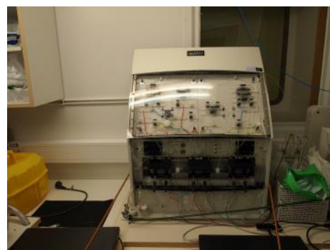
Continuous flow analyser QuAAtro from SEAL Analytical in the clean lab on ODEN. The instrument was used for continual on board measurements of nutrients in water throughout Leg 2.
