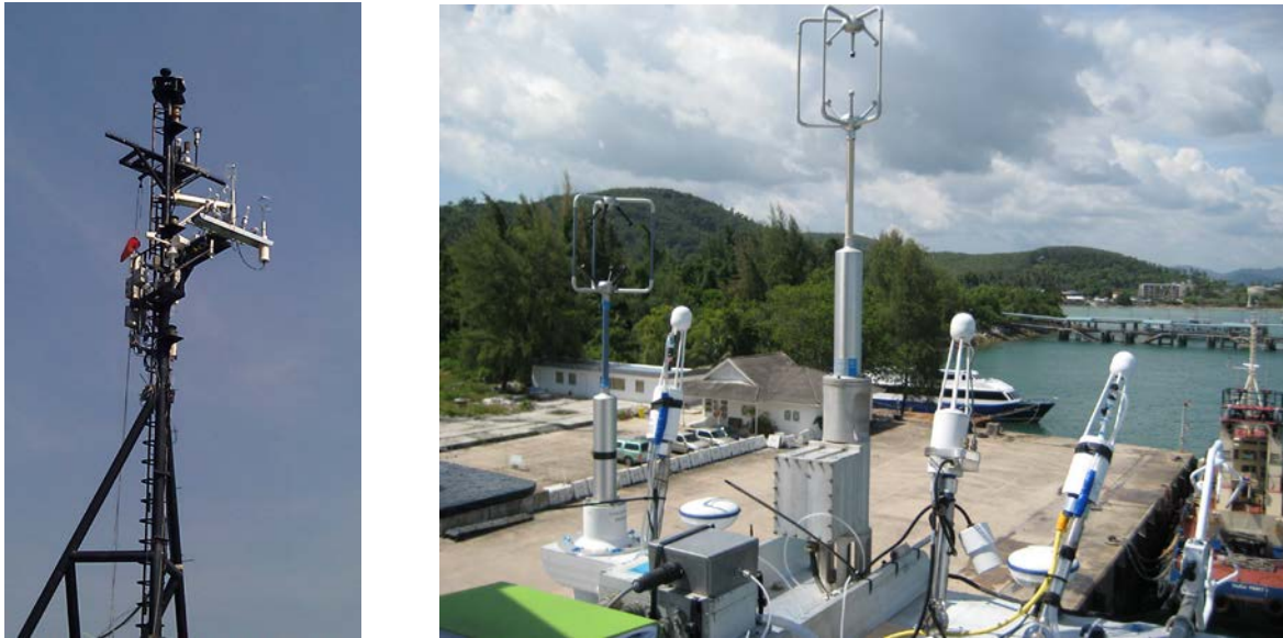
Figure 2. Views of the jackstaff and the PSD flux tower deployed on the R/V Moana Wave during STRATUS 2011.
