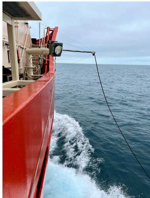
Figure 3: Sea snake position on the forward starboard-side railing. SST is recorded at 1 min -1 by a Campbell Scientific CR-1000 data logger located on the pilot house roof.
