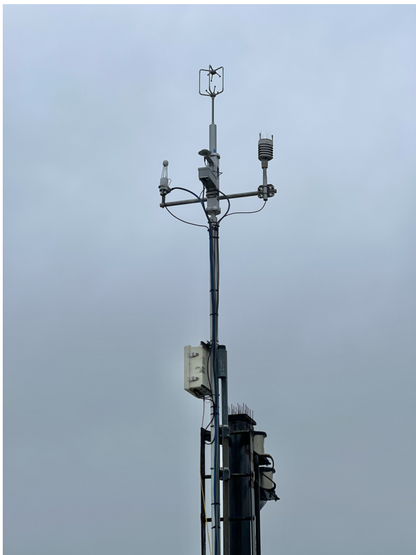
Figure 2: Bow mast installation: Gill R3A center top, LICOR 7500 on left, and Vaisala WXT on right. The IMU and GPS antenna are below the Gill R3. Height for the Gill R3A is 18.6 m ASL.
