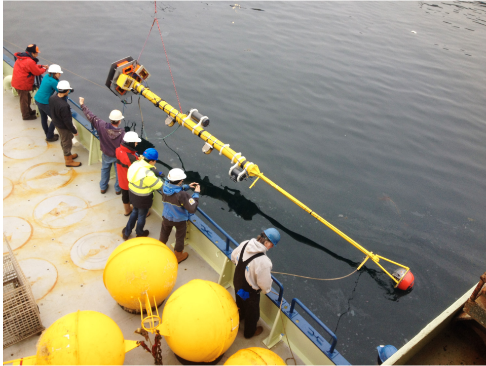
Figure 3: The large spar buoy with whitecap cameras, data acquisition and communication electronics at the top, wave wires and bubble-sizing instruments mounted along the length of the column, and batteries and sonar (upward looking) at the base.
