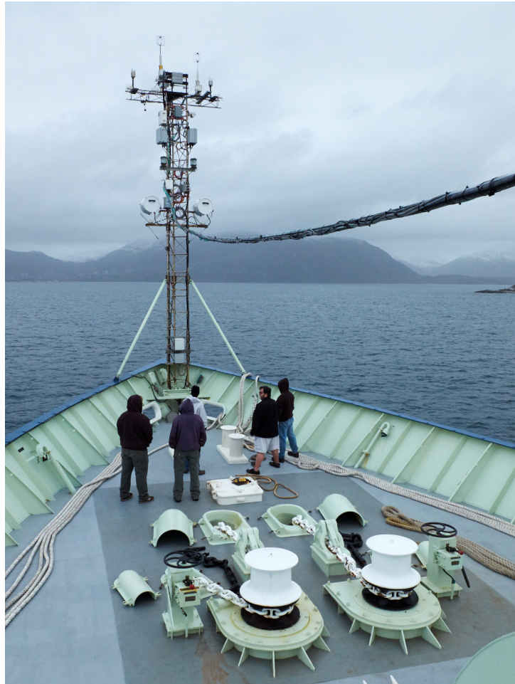
Figure 1: Bow tower installation for flux and bulk meteorological measurements.
