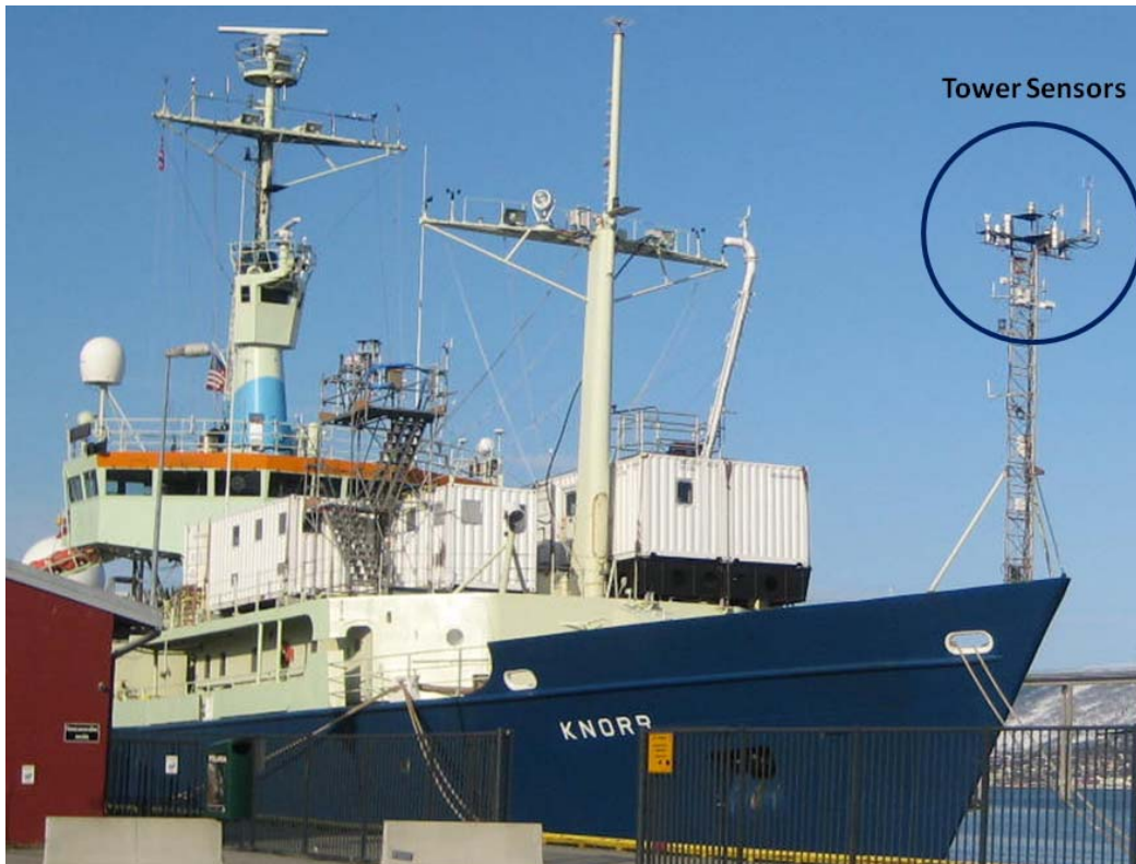
Figure 2. Tower sensors located on the forward mast on the bow of the Kno
