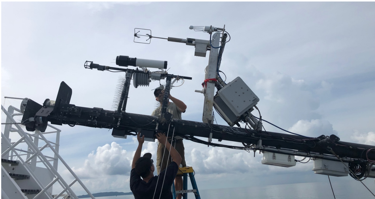
Fig 1: Ship and PSD met sensors at top of bow mast. Mast is lowered for access to sensors. PSD wind, T/RH, rain and fast water vapor sensors are ~ 0.5-1 m lower than the ship's SCS met instruments.
