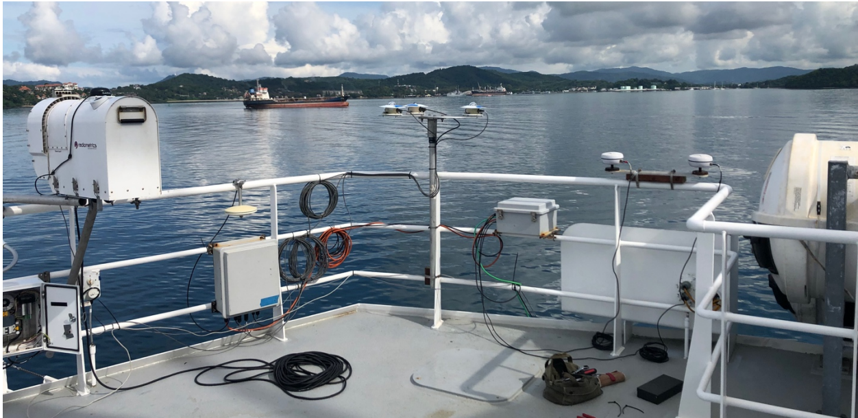
Fig 2: NOAA radiometers (center) and GPS/heading antennas (right) mounted on starboard side forward 02-level railing. The Notre Dame profiling radiometer is on the far left. The NOAA pressure sensor is inside the gray box just to the right of the profiling radiometer.
