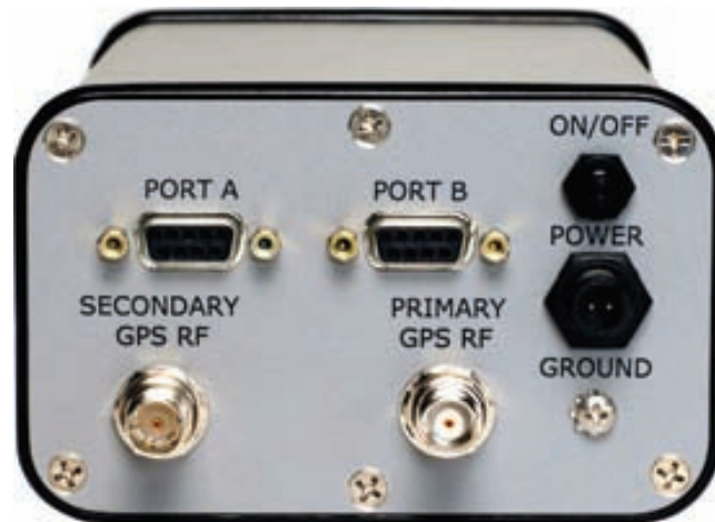
Figure 3-5. Turn the VS100 on at the Power toggle switch.
