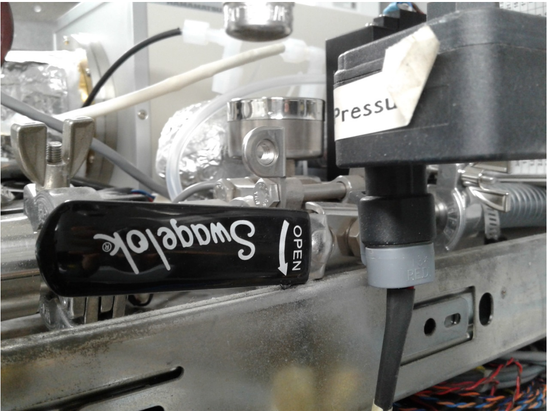
Pic 5: Second drawer: vacuum isolation valve.
