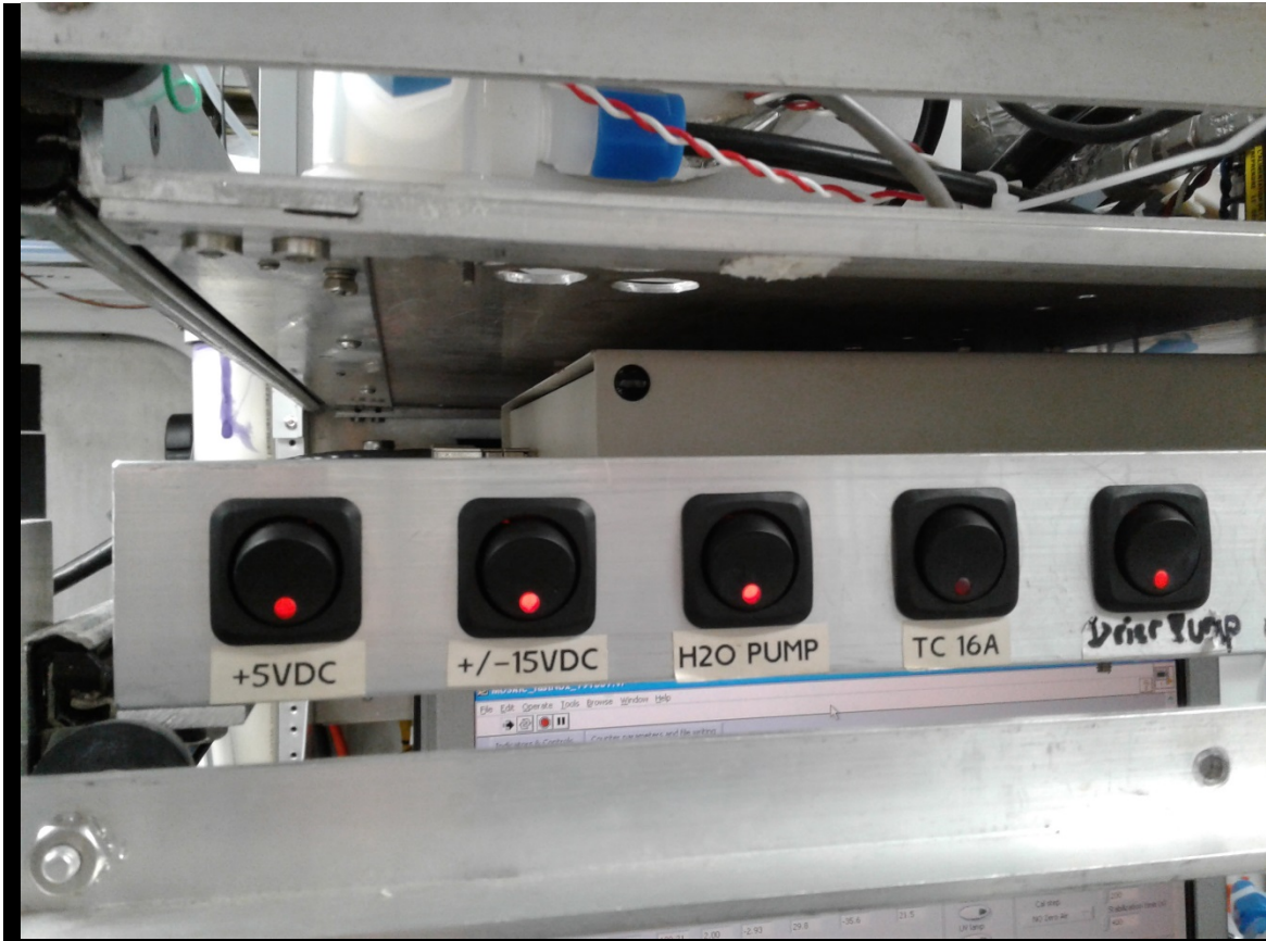
Pic 9: Second drawer: Main switches.
