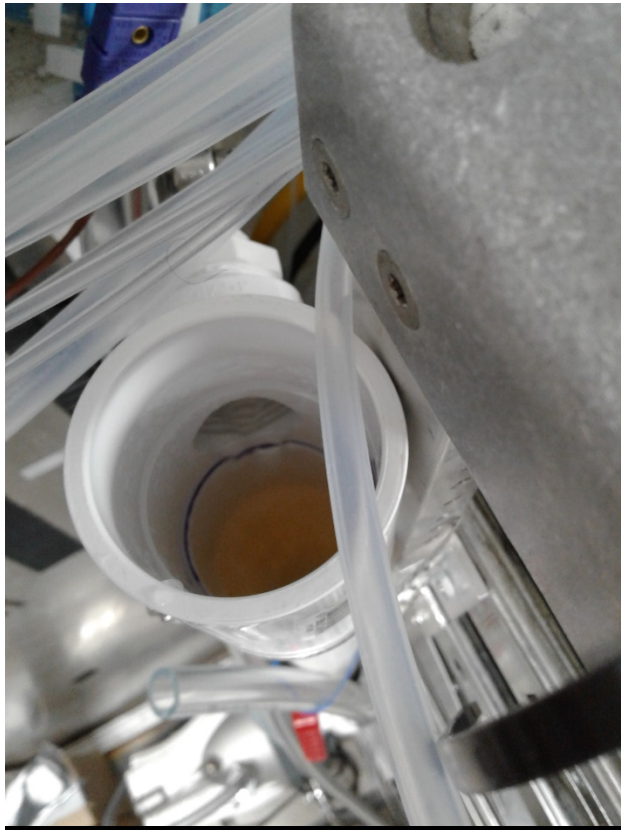
Pic 15: Water reservoir and water reservoir fill port
