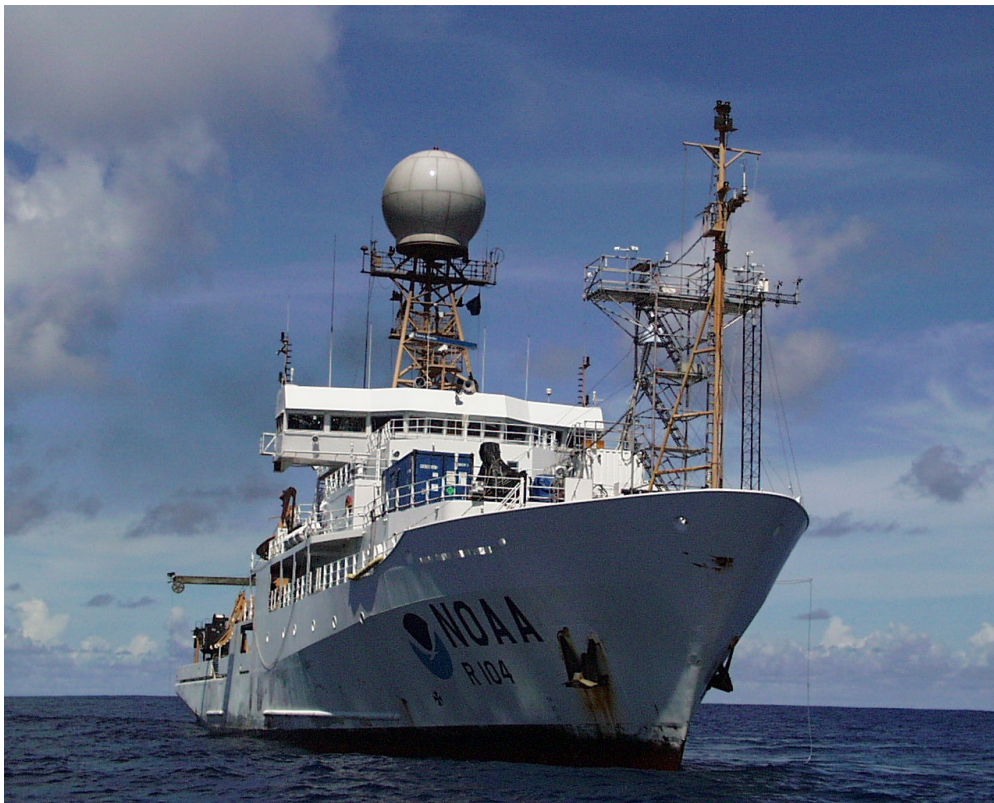
Figure 1 View of R/V Ronald H. Brown showing flux instruments on the bow tower and jackstaff. The large white sphere is the C-band Doppler radar.
