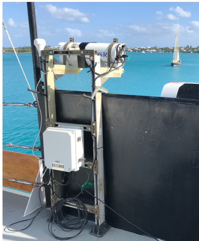
Figure 1: Experiment setup. The ROSR is mounted high on the ship (bridge roof) and, preferably on the port side. While underway, make visual confirmation that the view ( 9^\circ ) well outside the ship wake.
