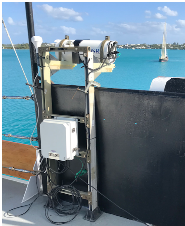
Figure 1: Experiment setup. The ROSR was mounted on the bridge roof, port side, approximately 9 m above the sea surface. While underway we made visual confirmation that the viewing field of view was well outside any ship wake.
