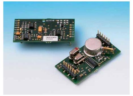
The Vaisala BAROCAP<sup>®</sup> Barometer Module PMB100 offers reliable barometric pressure measurement in a compact size.
