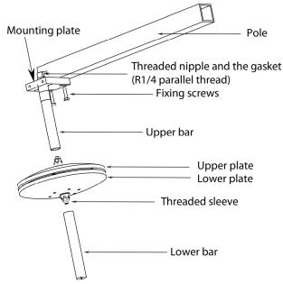
Figure 1 SPH10 Static Pressure Head
