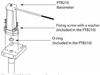
Figure 2 PTB210 Barometer Connection
