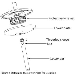
Cleaning the SPH10 is done by detaching the lower bar and the lower plate. The barometer can be in place while cleaning the
